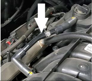
Rotate 90 degree rubber coupler towards front of engine.
